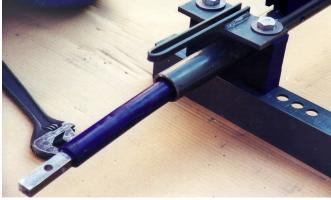
The Miller Tensioner is a steel spring tensioning device, encapsulated in polyurethane to protect it from contaminants. It controls scraper pressure on the belt and is located inside the scraper tube, reducing the space required for the scraper.
