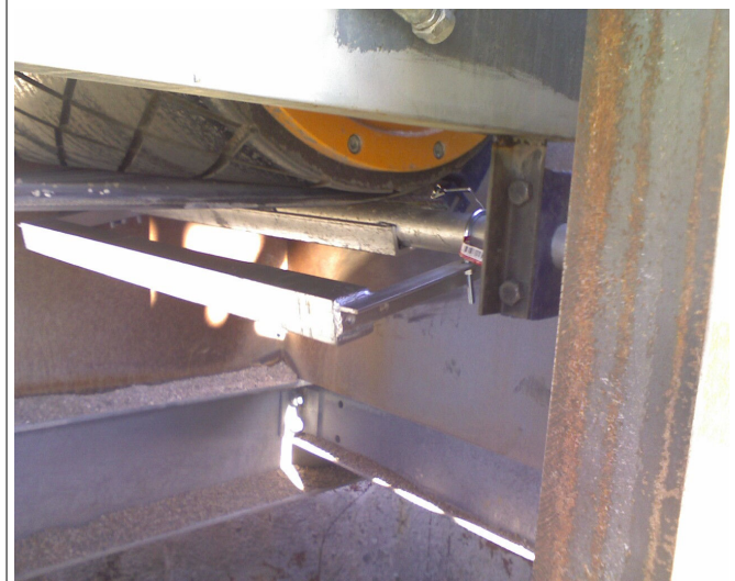
Counter-weight safely mounts under the belt!
