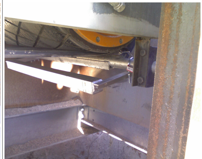
Counter-weight safely mounts under the belt!
